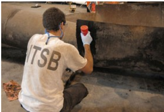
NTSB investigator examining fracture surfaces ( Download full-sized version )
