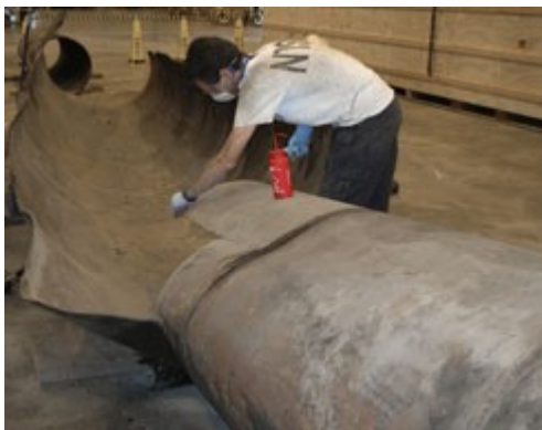
View of ruptured section of pipeline with investigator cleaning a fracture surface ( Download full-sized version )
