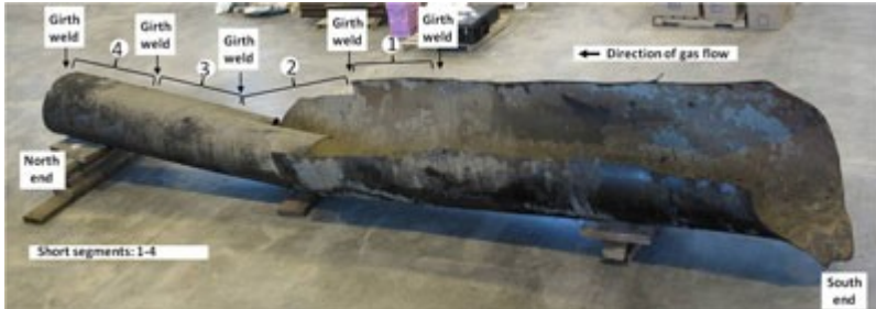
28-foot-long ruptured section of pipeline at laboratory facilities at the NTSB Training Center, Ashburn, VA ( Download full-sized version of image )
